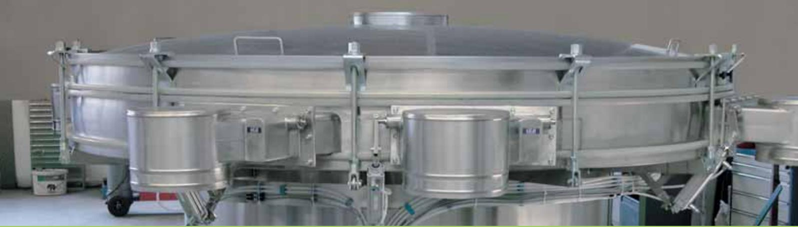
EA variable and easy selection of screen inserts with only a few fasteners, allows a fast adjustment to changed process conditions from 2 to 7 fractions within one machine with maximum screening efficiency.
