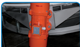
Driven by laterally attached vibration motors (ATEX 22)
